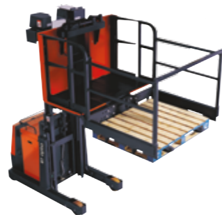
OME100 with auxiliary lift and OME100W walk-through version • Chassis width 970 mm • Maximum capacity 1000 kg • Picking heights to 3.35 m • Cabin widths 1000 mm, 1200 mm, 1400 mm
