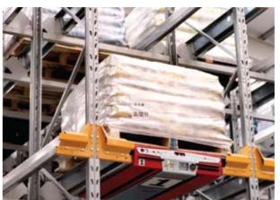
BT Radioshuttle units emit visual and audio signals when moving
