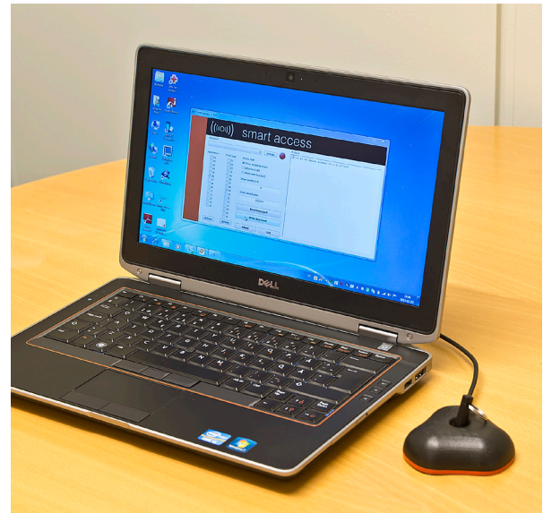
The ID-key is programmed through a programming unit which is connected to an ordinary PC.
