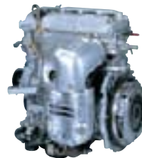
2AZ-FE gasoline engine (Displacement: 2.4 liters, used in the Estima)
