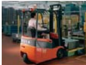
TRIGO Three-wheel electric counterbalanced lift truck (24V)
