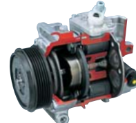
7SEU17 compressor (Swash-plate externally controlled, clutchless variable-displacement type)
