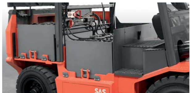
Easy 'lift out' battery extraction
